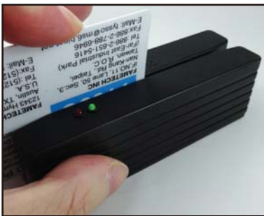
Reliable read head (up to 1,000,000 passes)
